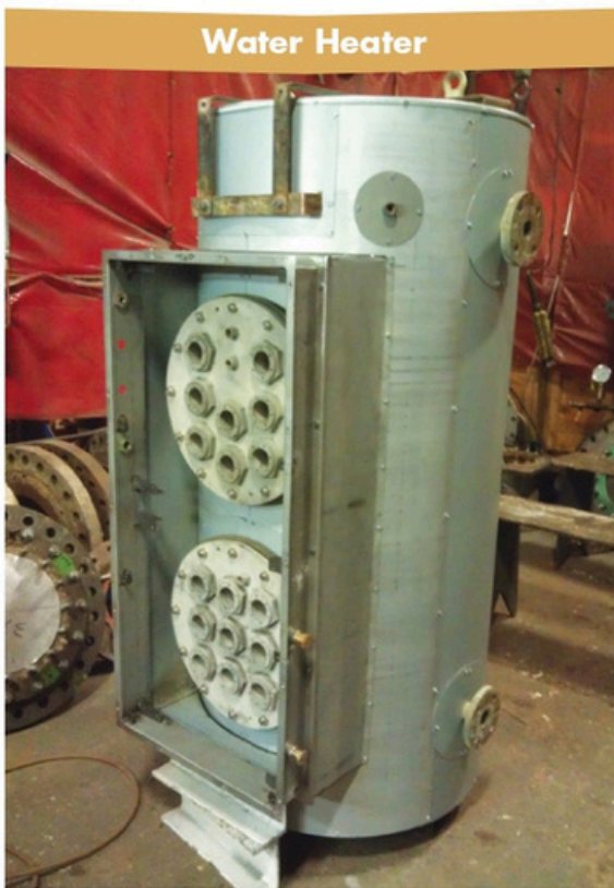
Admiralty pattern water heater during manufacture.
